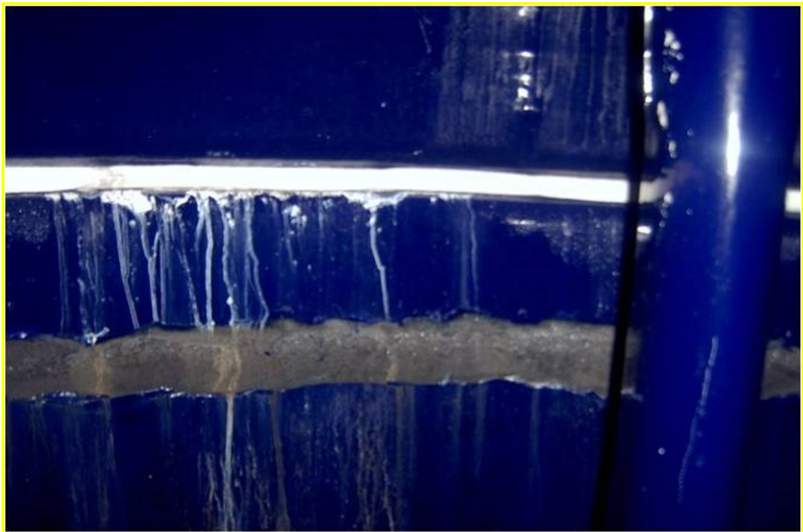
Pic.4 冷热温差急变引起的搪玻璃失效 Glass failure due to thermal shock/cold shock
